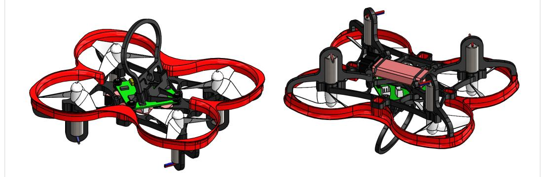
SPECIFICATIONS: Weight: Frame: 8.8g, total weight with FPV Camera mount: 10g Materials: Plastic. Size: 73mm. Maximum propeller: 40 mm. Motor mount: 7x20 mm. Flight controller mount: 29mm x 29mm.
